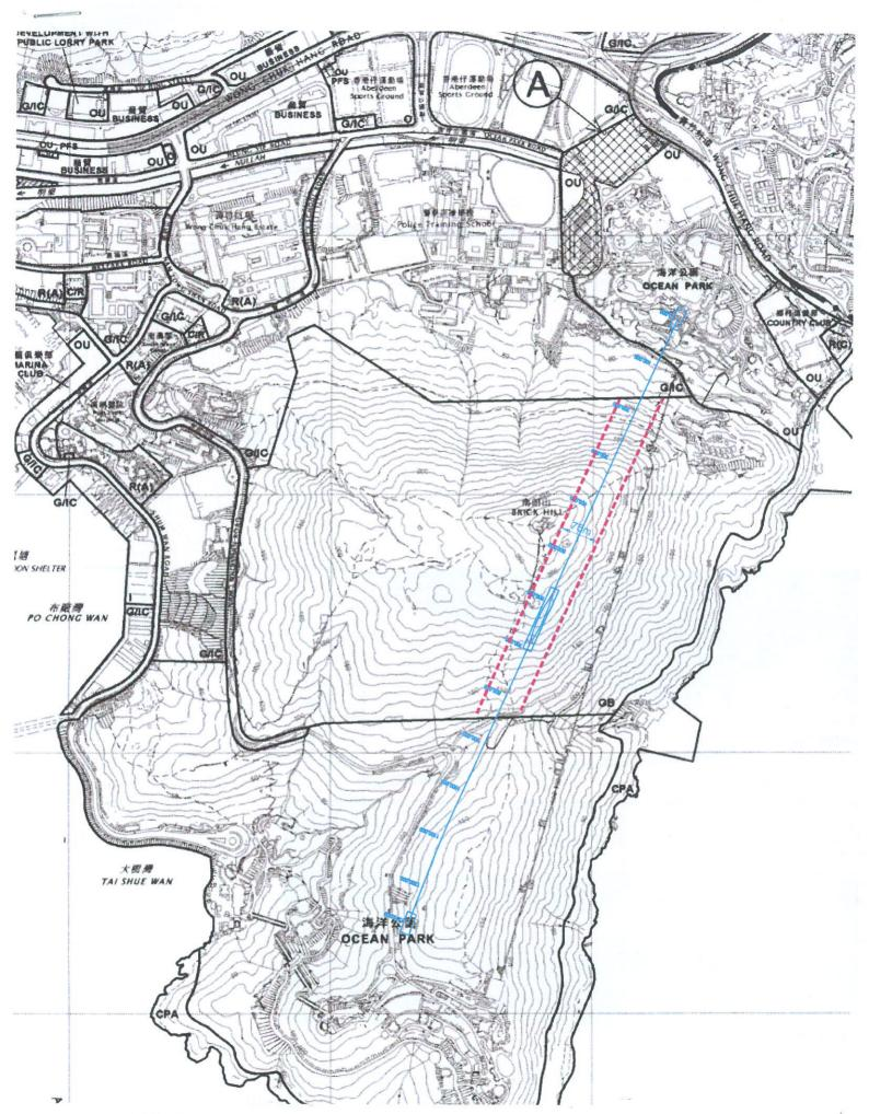
Figure S16-1 The Proposed Funicular Alignment and the Extent of Underground Reserve
